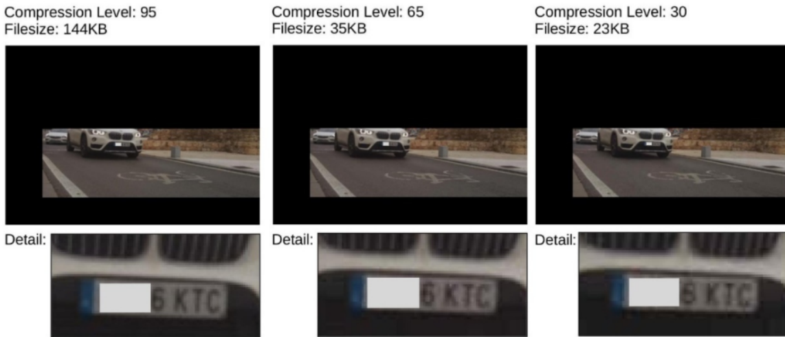
Figure 5.2: Images compressed with different JPG compression levels, with filesize data. Compression levels below 60 significantly compromise the ANPR success rate. The first three digits of the license plate are blurred for data protection [ÁBSCV+20]
