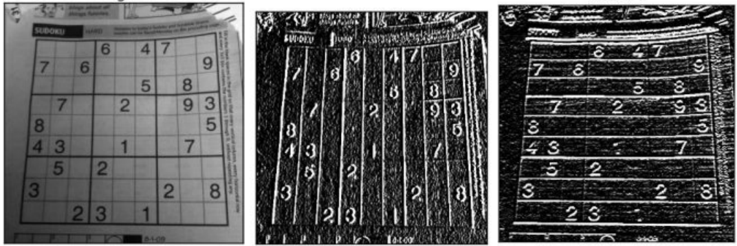
Figure 3.3: Example of application of the Sobel operator. From left to right: Original image, G_x , G_y . Source: OpenCV library documentation 4
